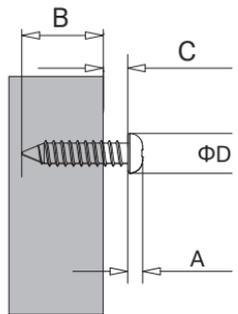
For a smooth installation, use screws with a diameter range of 4-8 mm for the screw cap
